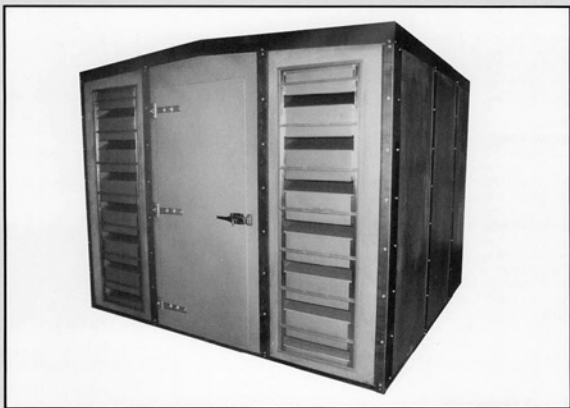
Fig. 5 Complete acoustic enclosure designed for 100 mph wind load with all wall and roof panels removable, tubular steel framework, sloped roof and acoustic louvers for air intake
